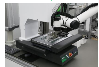
The robot automatically places the workpiece on the CNC vision measuring station for automatic measurement
