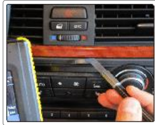
Measuring gaps on the car dashboard
