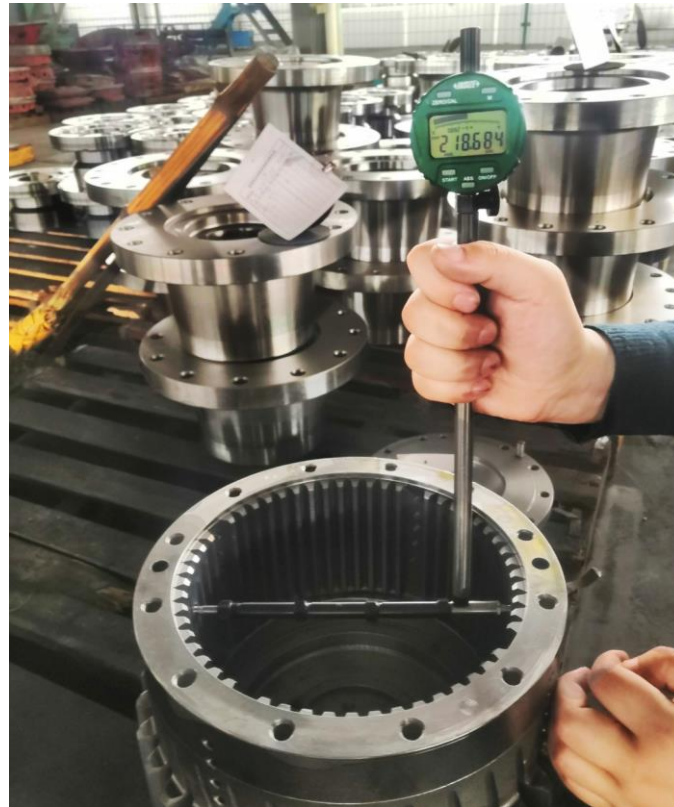
Measure the span measurement of the internal spline gear
