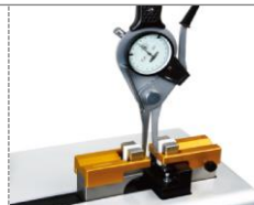
zero setting and calibration of internal/external snap gauges
