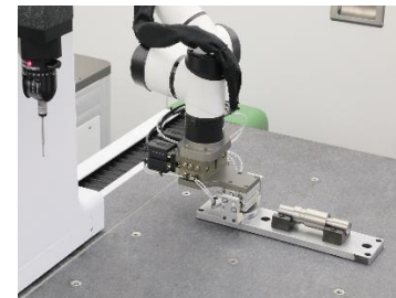
The robot automatically places the workpiece on the CMM station for automatic measurement
